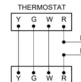
The Safety Float Switch may be used to provide additional protection against flooded drip pans by shutting-off the system that is producing the water or condensation in the event the pan floods, the pump's discharge becomes clogged, or other malfunction occurs. The switch may be wired to the thermostat circuit or it may be wired to any auxiliary alarm or other warning device.
